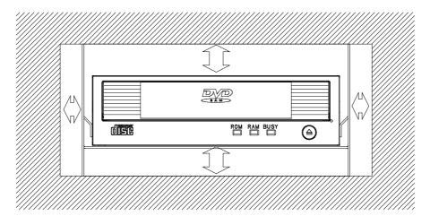
Keep more than 0.8mm clearance around the top cover in order to secure absorbing shock and vibration.
